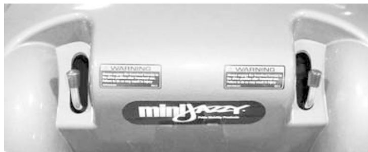
Figure 5. Freewheel Mode (Drive Motor Disengaged)
