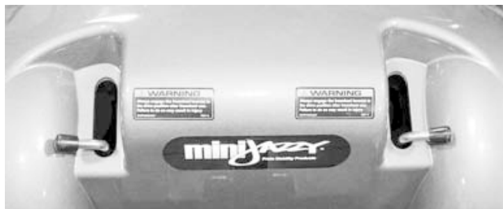
Figure 6. Drive Mode (Drive Motor Engaged)
